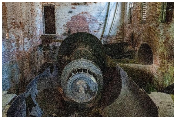
Industrial water turbine formerly used to power Building 13
