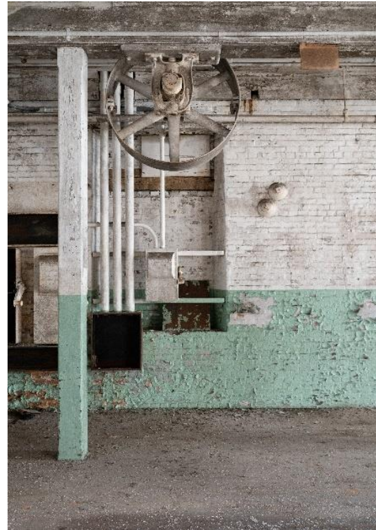
Flywheel formerly connected to water turbine in Building 13
